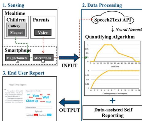
Figure 2. System Block Diagram of MAMAS
